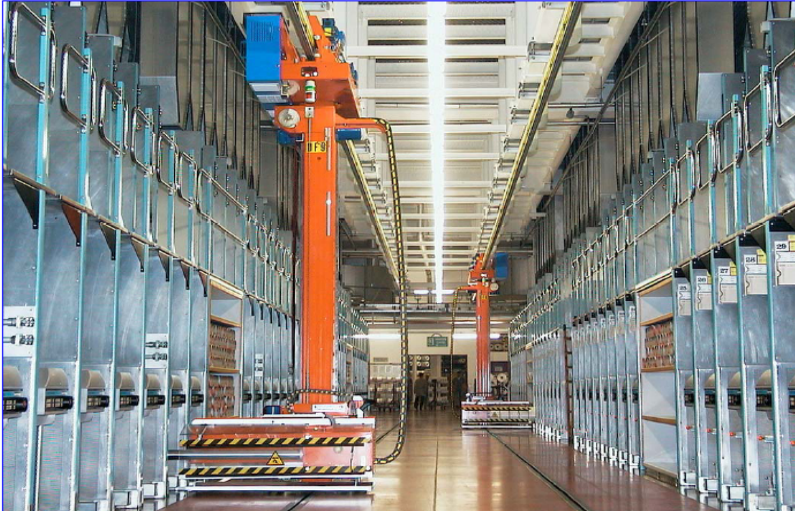
Salmoiraghi Automatic Doffers in operation
